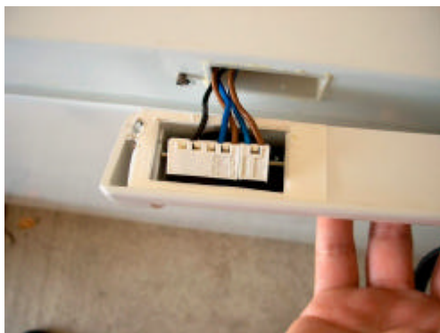
10. Fit the new PCB to the handle and plug in the new connectors
