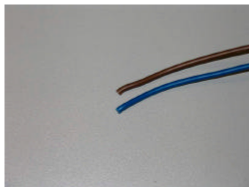
10. Cut the plug-in terminals from the end of the lamp wires
