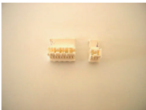
8. Take the new connector (in the kit), open its cover and remove the empty driving pins
