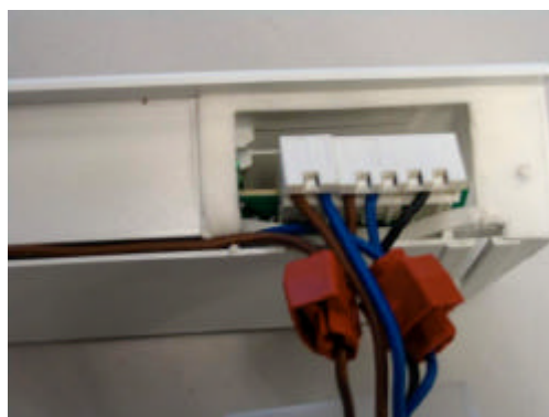
13. Put the PCB into the handle, connect the 5 and 2 pole connectors to the PCB, push the lamp wires in their place and reassemble the handle.
