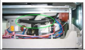
Fig. (1): Hose is sagging Fig. (2): Serial solution
