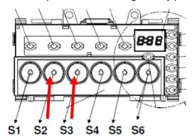
On EDW3000 user interface family: Pressing buttons S3+S4 at least 1sec or - as well single button when specified on according PNC by personalisation
