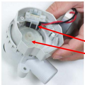
Washer with three holes to switch the Different water flow ways
