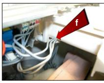
After releasing the wiring from the fixing hooks.
