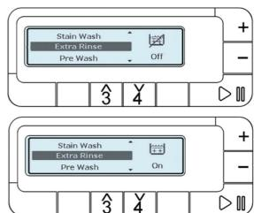
After 2 seconds the writing changes to "PUSH OK"; pushing button **5** it is possible to change the option state from active to inactive or vice versa.
