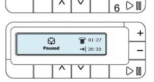
If the phase of the washing cycle which includes a pause corresponds to a condition by which the door can be open, the display will show the relative symbol.
