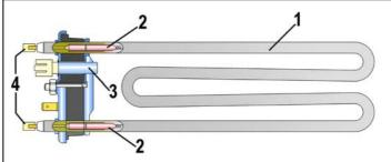
The heating element is powered by a relay (K1) of the electronic board and is provided with two thermal fuses, which interrupt if the temperature degree exceeds the values by which they are calibrated.
