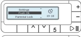
It is possible to modify the time with buttons 3 or 4. Pushing it in sequence the time increases or decreases (respectively with button 3 and 4) by thirty minutes for the first two hours and sixty minutes till the twenty hours are reached (the max. time available for the delayed start).
