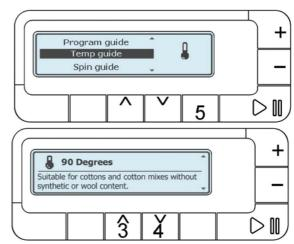
Waiting some seconds or pushing buttons: TEMPERATURE (1) or SPIN (2) or START/PAUSE (6) the main screen is displayed again.
