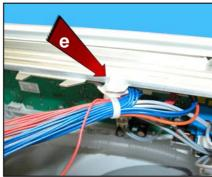
f. Release the wiring from the clamp under the dispenser.
