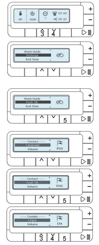
Waiting some seconds or pushing buttons: TEMPERATURE (1) or SPIN (2) the main screen is displayed again.
