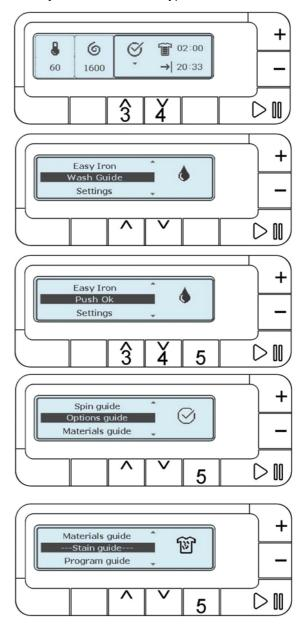
Waiting some seconds or pushing buttons: TEMPERATURE (1) or SPIN (2) or START/PAUSE (6) the main screen is displayed again.
