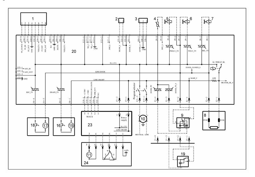
• Key to diagram WM with THREE-PHASE ASYNCHRONOUS MOTOR EWM 25xx
