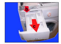
d. Remove the screw which secures the control panel to the dispenser.
