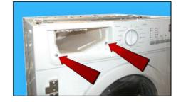
d. Remove the 3 screws which secure the cross-member to the cabinet and the conveyor.
