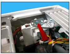
g. Remove the 2 screws which secure the control panel to the cross-member.
