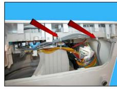
I. If problems with the door microswitch wiring should arise, detach the connector from the board.
