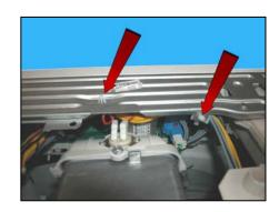
h. Remove the screw which secures the PCB (which controls the WD section) to the bracket, extract it and position it so as it does not interfere with the disassembling of the control panel.
