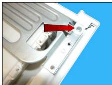
h. Release the 2 hooks (one on the right, the other on the left) which secure the control panel to the cabinet.
