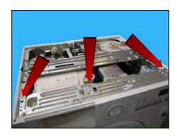
e. Release the wiring supports from the cross-member.
