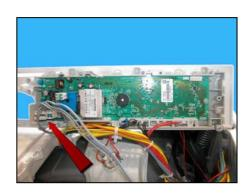
m. To extract the board unscrew the screws, release the hooks which fits it to the control panel.
