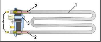
The heating element is powered by a relay (K1) of the electronic board and is provided with two thermal fuses, which interrupt if the temperature degree exceeds the values by which they are calibrated.
