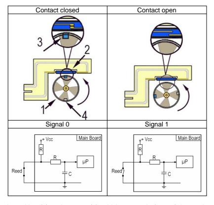
Water entering the solenoid valve rotates the turbine (1) and magnet (3), which passes in front of the reed switch (2), thus closing it. As this contact opens and closes, it generates pulses at a frequency that is a function of water flow.
